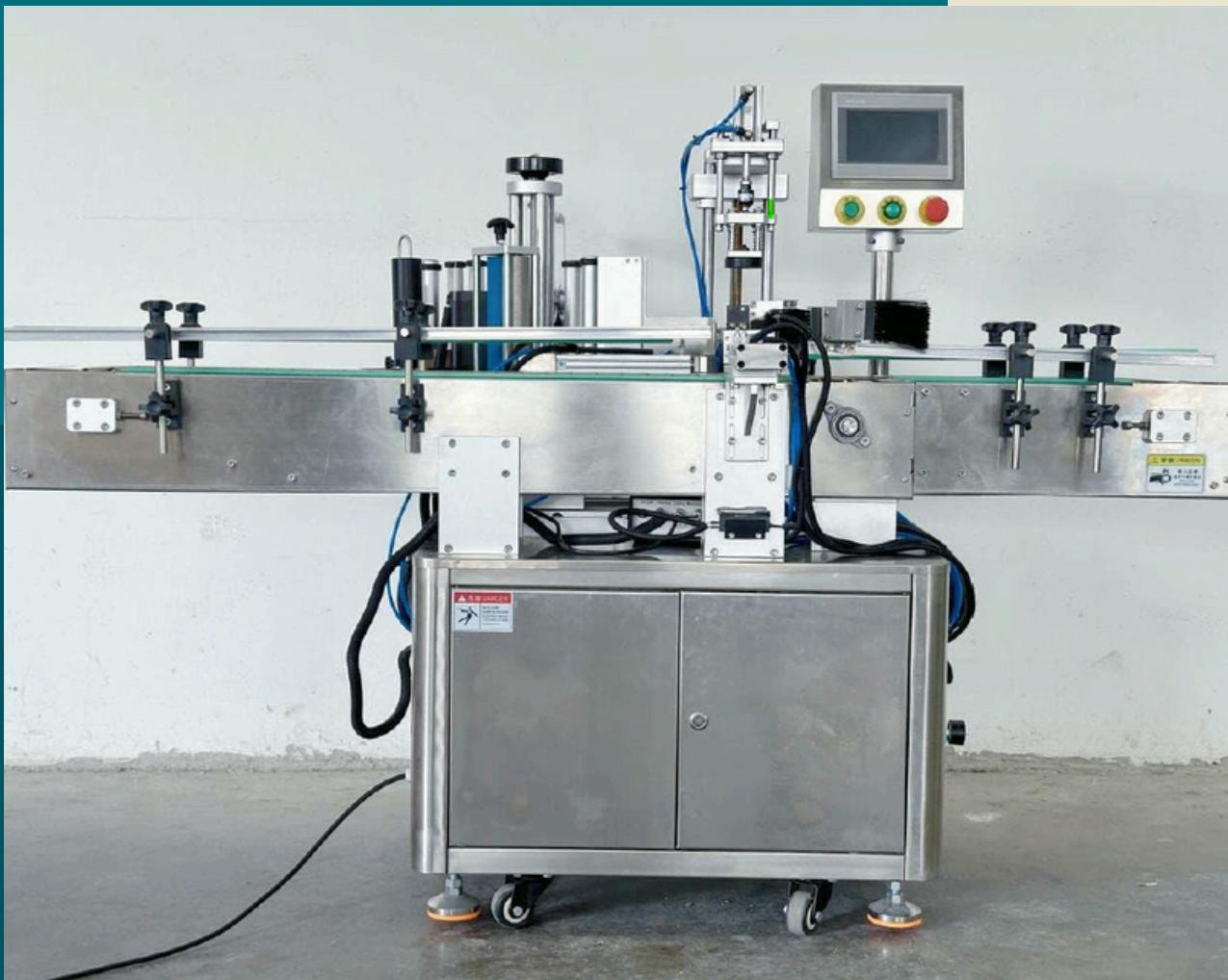
**XLE-300** Fully Automated Labeling System for Square Bottles. The **XLE-300** is a fully automated labeling system engineered to deliver accurate, consistent, and high-speed labeling for square bottles. Designed for modern manufacturing environments, it ensures maximum productivity, stable operation, and premium labeling quality.
